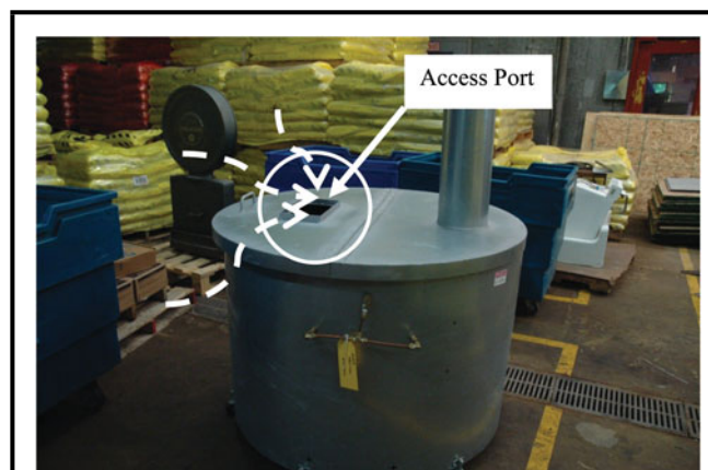
FIGURE 2. Hinged lid-closed hood and exhaust configuration in test room (access port is shown) used in study. Note: Dashed arrows reflect airflow into the mixing tank (color figure available online).
