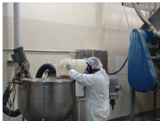
FIGURE 1. Flavoring ingredients manually added to the mixing tank with a ventilated lid through an access port at a flavorings plant (color figure available online).
