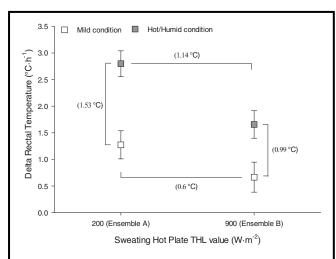
**FIGURE 4.** Changes in rectal temperature during human testing (Values are mean and standard deviation. Values in parentheses indicate mean difference in rectal temperature between trials.)
