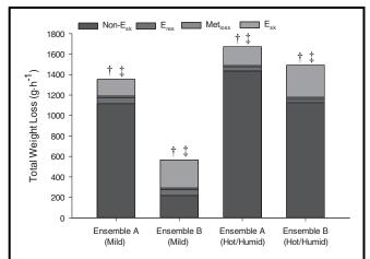
**FIGURE 2**. Total weight loss during human ensemble testing (stacked by each weight loss element) (Values are mean. Non-E<sub>sk</sub>: non-evaporative sweat loss, E<sub>res</sub>: evaporative loss through respiration, Met<sub>loss</sub>: metabolic weight loss due to O<sub>2</sub>/CO<sub>2</sub> exchange, and E<sub>sk</sub>: evaporative sweat loss. Symbols denote a statistical difference (p < 0.05) between ensemble A and B in E<sub>sk</sub> (†) and Non-E<sub>sk</sub> ( $^{\ddagger}$ ).)
