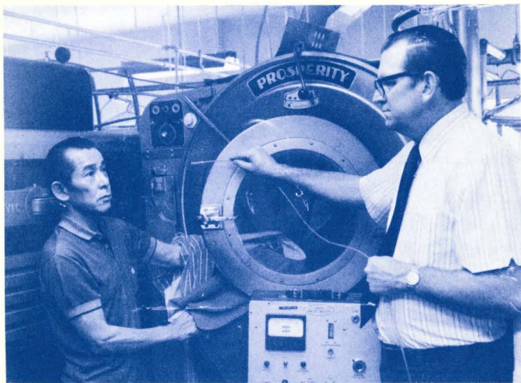
Lee Larson, of WAOHL staff, samples the air at the dryer door as Sam Watanuki removed dried clothing in a Salt Lake City dry cleaning shop.
