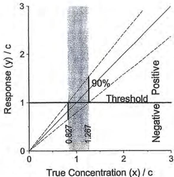
Figure 3 A quantitative method with  $A = 0.25$  and converted to qualitative outcomes (positive or negative with respect to a threshold level) by use of a threshold value.
