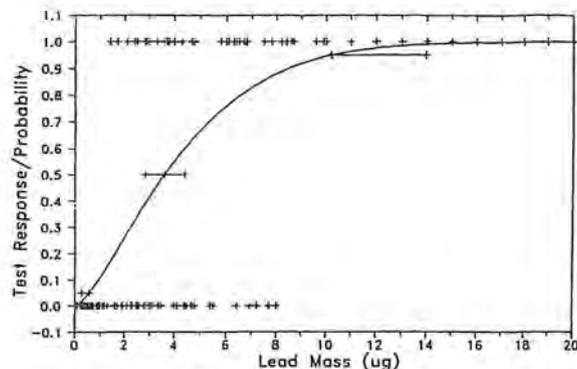
**Figure 5** Data fitted by statistical modeling: lead spot test applied on workplace air filter samples.<sup>1</sup> Plot of spot test response/probability versus mass of lead per filter (determined by GFAAS). +: individual data points; —: modeled performance curve.
