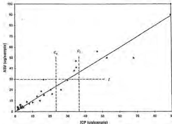
**Figure 7** Plot of data obtained by portable UE/ASV versus ICP-AES results for lead in workplace air samples.<sup>23</sup>
