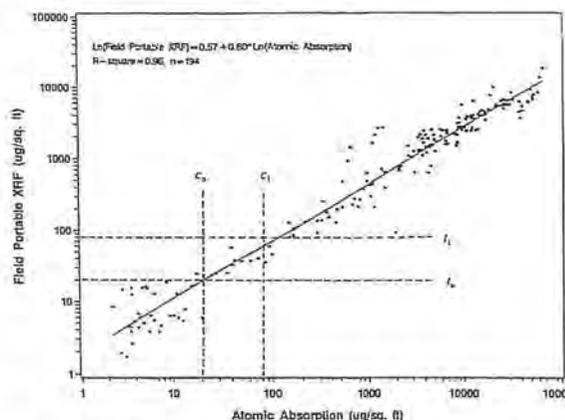
**Figure 6** Plot of field-portable XRF data versus GFAAS results for lead in dust wipe samples.<sup>17</sup> (Courtesy of D.T. Woody and Prof. C.S. Clark, University of Cincinnati.)
