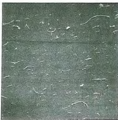
FIGURE 25-1. Scanning Electron Micrograph (1500 \times ) of an Aqueous Sample of Magnetically Aligned UICC Canadian Chrysotile Collected on a 0.1 \mu\text{m} Pore Size Filter. (Source: Timbrell 1973.)
