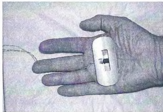
FIGURE 5. The palm-held adapter recommended in ISO-10819, 1996 (from Ref. 122).
