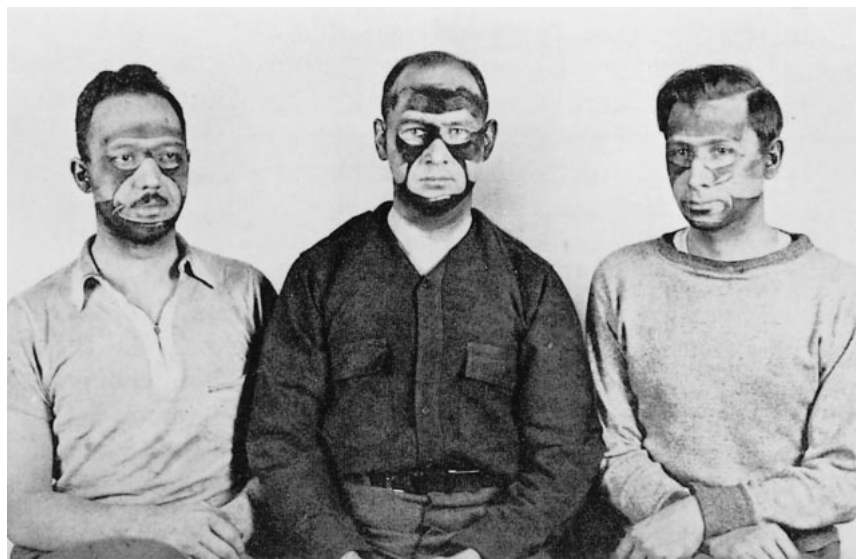
FIGURE A1. Coal dust deposition pattern on the faces of subjects after wearing half-facepiece respirators in the “coal dust tightness test” conducted by the former Bureau of Mines as part of its respirator certification program from 1934 until 1972. Only the center subject shows no leaks. The other two show leaks induced during a demonstration by a toothpick under the facepiece. Many facepieces submitted to the Bureau of Mines had to be redesigned before they could meet fitting requirements. (17)
