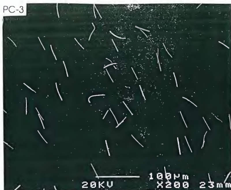
FIG. 2b—A picture of glass fibers produced with the fiber length classifier
