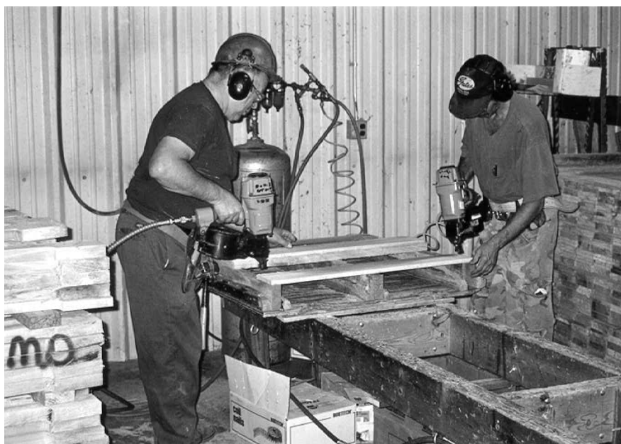
FIGURE 1 Employees of a sheltered workshop using pneumatic nail guns to make wooden pallets.
