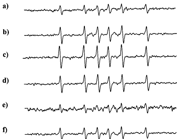
Figure 3. ESR spectra of 2a with and without NAC or aspirin. All spectra were recorded on samples dissolved in phosphate buffer (100 mM, pH 7.4) and DMPO (20 mM) and (a) 2a (2.0 mM) immediately after mixing, (b) 2a (2.0 mM) after 15 min, (c) 2a (2.0 mM) added to NAC (2.0 mM) immediately after mixing, (d) 2a (2.0 mM) added to NAC (2.0 mM) after 15 min, (e) 2a (2.0 mM) added to aspirin (2.0 mM) immediately after mixing, and (f) 2a (2.0 mM) added to aspirin (2.0 mM) after 15 min. In all cases, the concentrations refer to the final concentration. All spectra were recorded under identical spectrometer settings.
