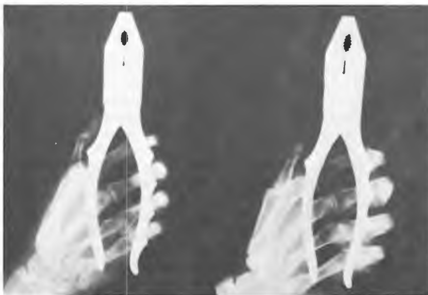
Figure 22.34 Form-fitting grips on hand tools may cause severe pressures on the finger joints of a person with a larger hand than the hand size for which the tool was designed. From Reference 46, by permission. © Journal of Occupational Medicine, Chicago, Ill.
