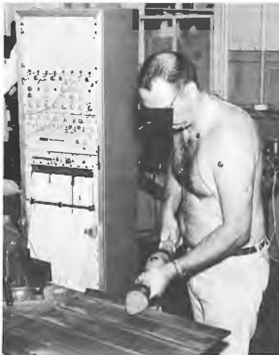
Figure 22.17 The recording of surface electromyograms by means of a commercially available oscillographic recorder for the purpose of physiological work measurement.
