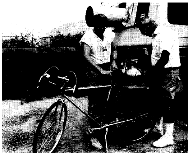
Fig. 1. Preparation of a Summa canister to collect air sample along an open path infrared beam at an industrial site fenceline in Delaware in 1988. The canister was transported along the beam path at a constant speed using the bicycle, thus obtaining a beam path averaged concentration sample. Shown are R. d'Simone (left) of MDA Corporation and Dr. G. Russwurm of ManTech Environmental. Dr. Russwurm was the cyclist. The instrument telescope is visible in the center.
