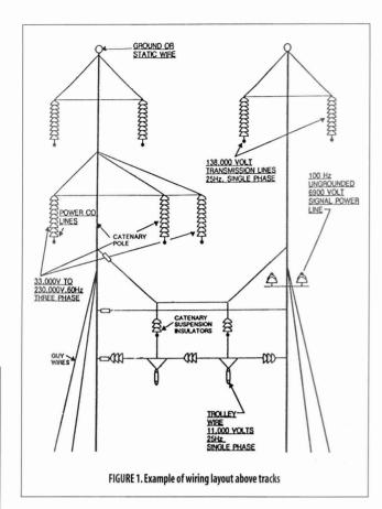
generated by electric current flowing in two different but related circuits near the tracks. To power the train, 25-Hz current flows from the catenary to the train and returns through the rails, completing the circuit in a loop varying from 6 to 10 miles in length (Figure 2). Higher on the poles, other 25-Hz current flows continuously in the high-voltage transmission wiring, which supplies a much wider area.
