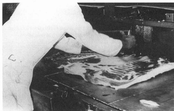
Figure 8. The worker uses a special knife to pull ribs. The design of the knife requires that the worker's thumbs be placed up on the handle to overcome mechanical disadvantages.
