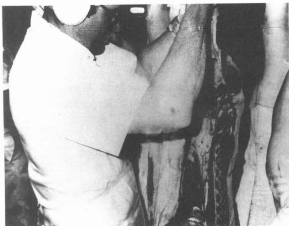
Figure 3. Near completion of the task, the worker's hands are at approximately head height. The shoulders are flexed to almost 90°. The tissue is easier to tear during this phase of the task.
