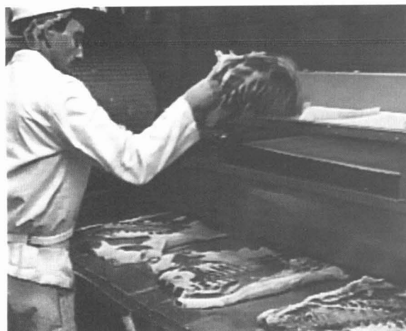
Figure 11. To set the ribs on the aside conveyor properly, they must be turned over. As a result, the worker pronates the forearm just prior to placement. Note that the aside conveyor is elevated and away from the worker, thus requiring shoulder and trunk flexion to reach it.
