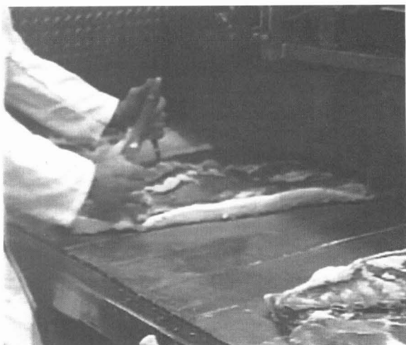
Figure 9. The distal end of the bellies are held in place by a spike conveyor. The worker reaches to the far end of the belly to start the cut. The knife slides under the ribs.
