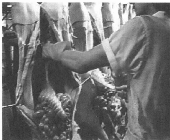
Figure 4. At the beginning of the work cycle, the Gut Snatcher reaches up to wrap the bung around the hand, then pulls down to free the rectum from the abdominal wall.
