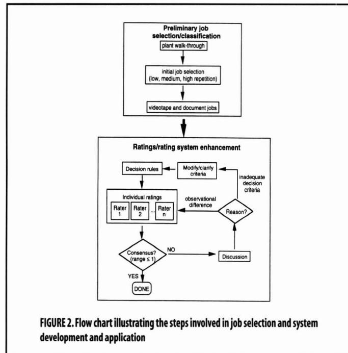
FIGURE 2. Flow chart illustrating the steps involved in job selection and system development and application
