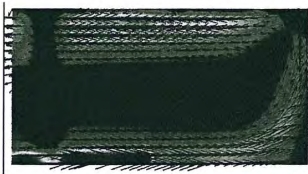
Figure 2: Velocity vectors and contours from PIV experiments for 30 Foot Slab Cut
