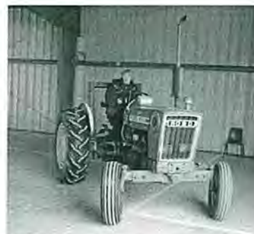
Figure 8 Driving the NIOSH AutoROPS Equipped Tractor
