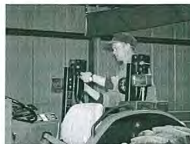
Figure 6 Lowering Manually Adjustable ROPS
