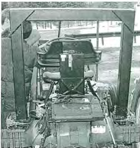
Figure 1 NIOSH AutoROPS 3rd Generation Design
