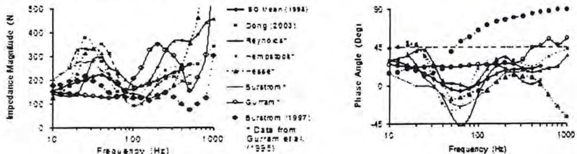
Figure 1 A comparison of several typical sets of MI data (in Z_h -direction) reported in the literature.
