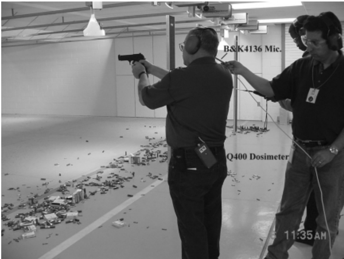
FIGURE 2. Personal noise exposure measurement
