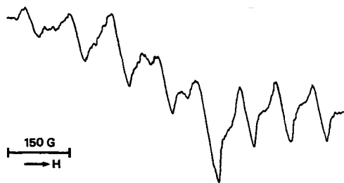
FIGURE 1. (a) ESR spectrum recorded 52 minutes after mixing in a phosphate buffer solution (pH 7.2) of 2.5 mM \text{NaVO}_3 , 2.5 mM NADPH and 15 units/ml glutathione reductase. The reactants were stirred in a test tube under ambient air for 52 minutes and then a small droplet was transferred to a 5 mm o.d. NMR sample tube for the ESR measurement.
