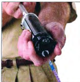
Sorbent tube samplers for workplace gases and vapors are used in a number of standards developed by Subcommittee D22.04.
