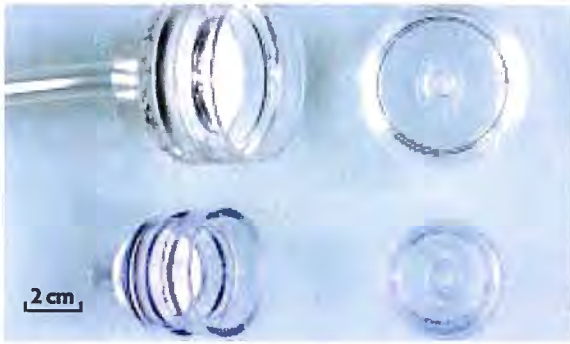
Examples of Filter Samplers Used in ASTM Methods for Collecting Workplace Aerosols in Order to Monitor Worker Exposure.
