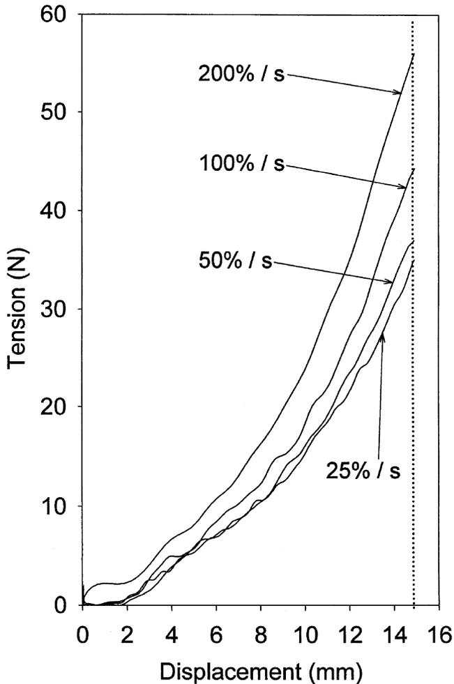
Fig. 4. The length–tension relation of a ligament when stretched at different rates. Increasing the rate of stretch from 25%/s to 200%/s develops nearly 50% more tension in the supraspinous ligament [13].
