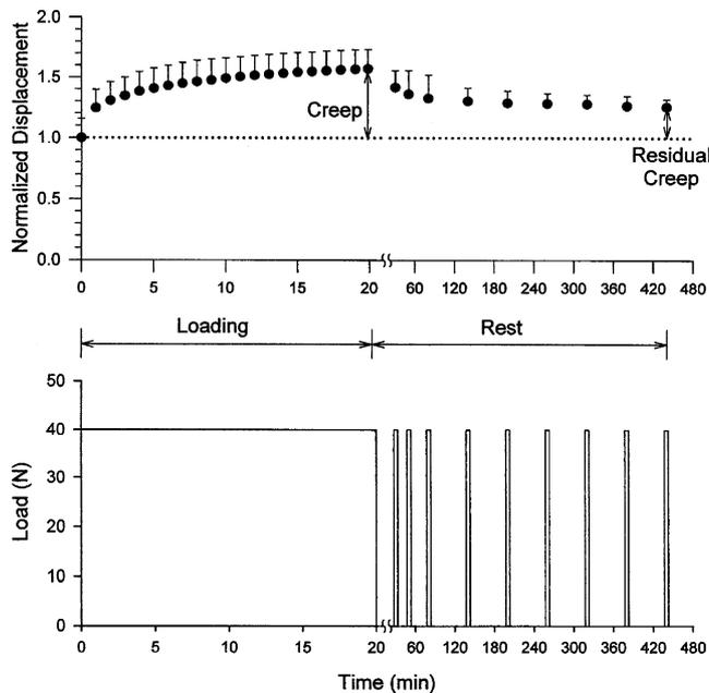
Fig. 2. The response of the supraspinous ligament to a constant load applied for a 20 min period exhibit the development of creep. The recovery during 7 h rest was not complete. In the rest period, short (6 s) loading tests were applied to determine the residual creep [72].
