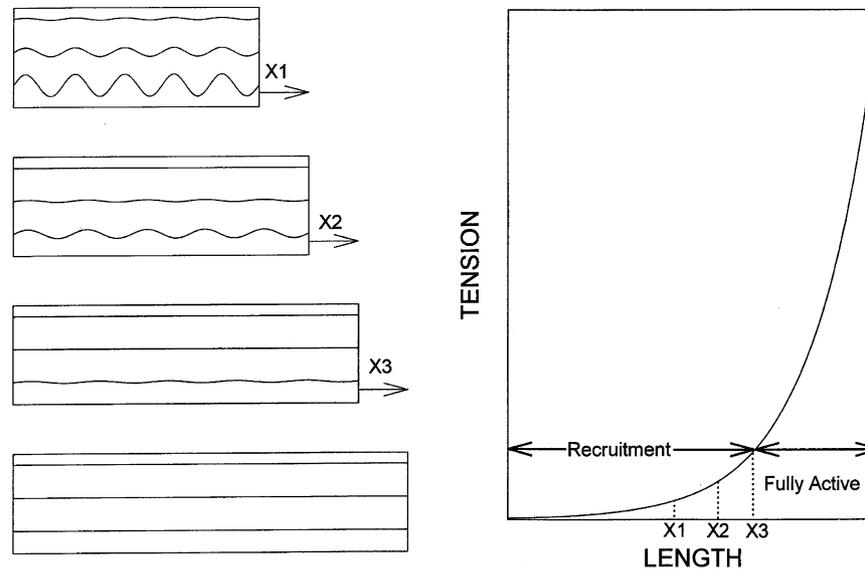
Fig. 1. The length–tension behavior of a ligament is shown on the right. On the left, the progressive recruitment of collagen fibers is shown for several elongations.
