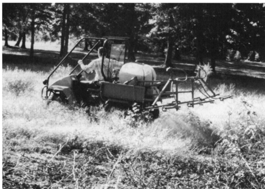
FIGURE 1. All-terrain vehicle with a spray boom operated by a USDA PPQ officer to apply paraquat to a field infested with witchweed.
