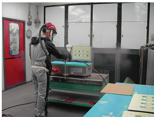
2 Permeation panel II set-up. Modified panel is mounted in its reciprocating arm, in line with the spray gun that is fixed at the front of the unit. The painter triggers the spray gun to apply clear coat as the panel moves left to right.
