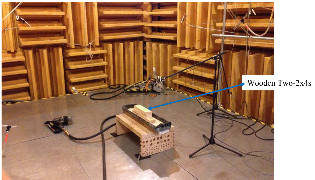
Figure 3 – Test setup. Wooden Two-2x4s are stacked in the sand box to receive the nails.
