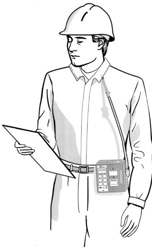
Figure 2 Personal air sampling train attached to a worker. Provided courtesy of SKC Incorporated, used with permission.
