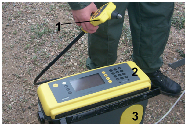
Figure 7 Hapsite™ person-portable GC-MS instrument deployed in the field. (1) Sample collection probe; (2) control keypad on instrument faceplate; and (3) interface for attachment of the instrument to a servicemodule containing mechanical vacuum pumps (service module usable only when AC power is available). From Smith et al. 88 Copyright (2004), with permission from Elsevier.
