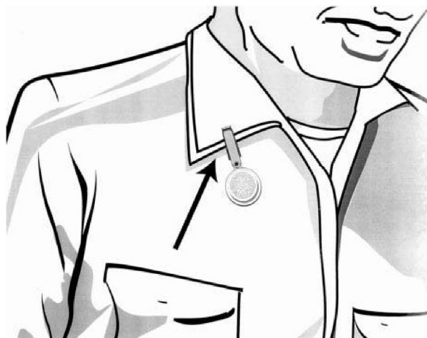
Figure 4 Diffusive sampler attached to a worker. This method is more acceptable to workers but the uptake rate varies from chemical to chemical and cannot be altered by field hygienists. Provided courtesy of SKC Incorporated, used with permission.
