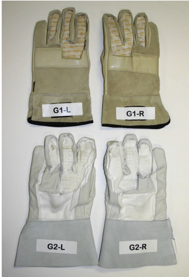
Fig. 4. Four tested gloves, two for each of the two models: Glove 1 is a gel-filled vibration-reducing glove; Glove 2 is air bladder-filled vibration-reducing glove.
