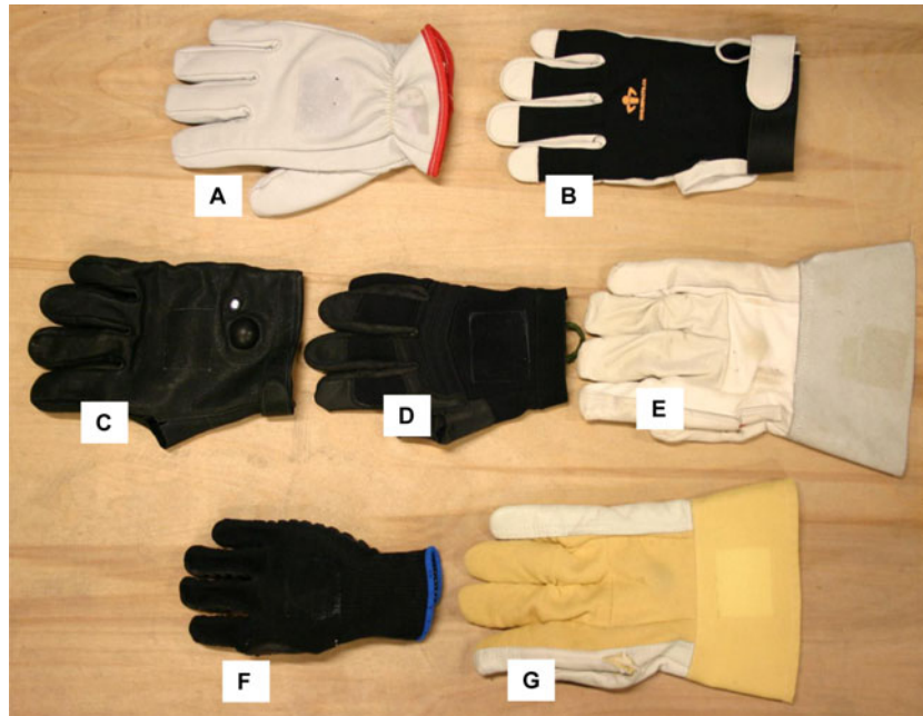
Figure 1. Seven glove models were evaluated in the study. Models A–C and E–G were VR gloves while Model D was an ordinary synthetic leather work glove.
