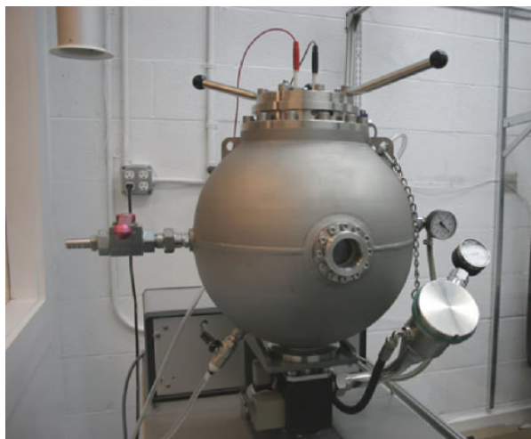
Figure 3 Siwek 20-L chamber.
