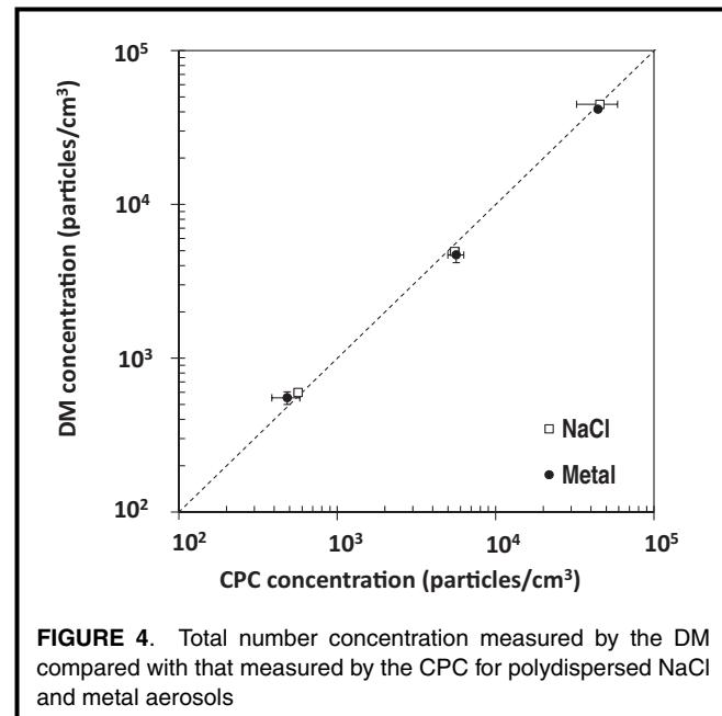
**FIGURE 4.** Total number concentration measured by the DM compared with that measured by the CPC for polydispersed NaCl and metal aerosols
