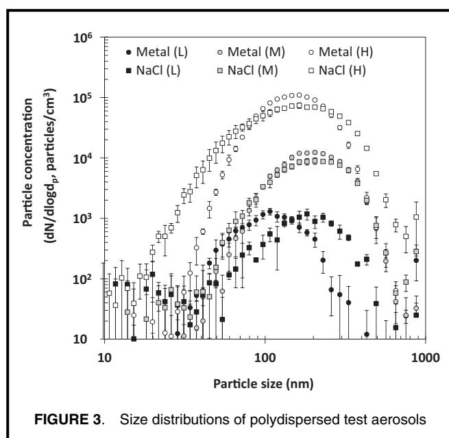
**FIGURE 3.** Size distributions of polydispersed test aerosols
