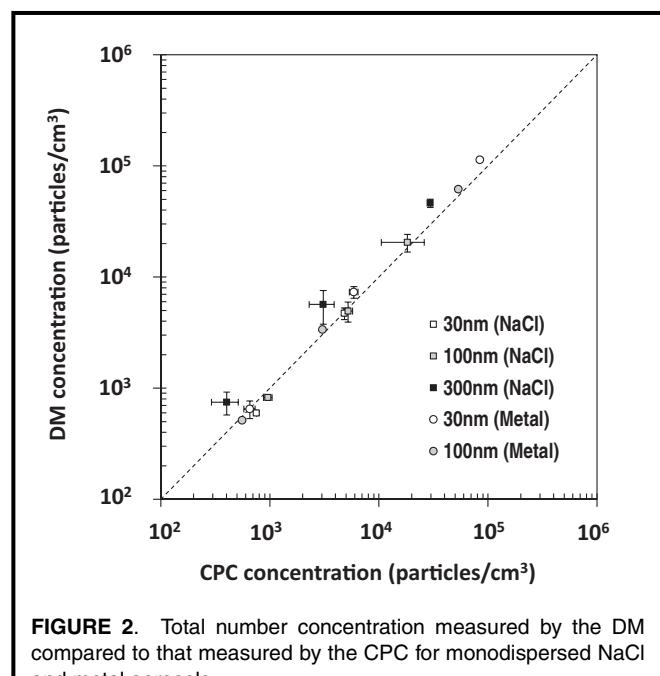
**FIGURE 2.** Total number concentration measured by the DM compared to that measured by the CPC for monodispersed NaCl and metal aerosols
