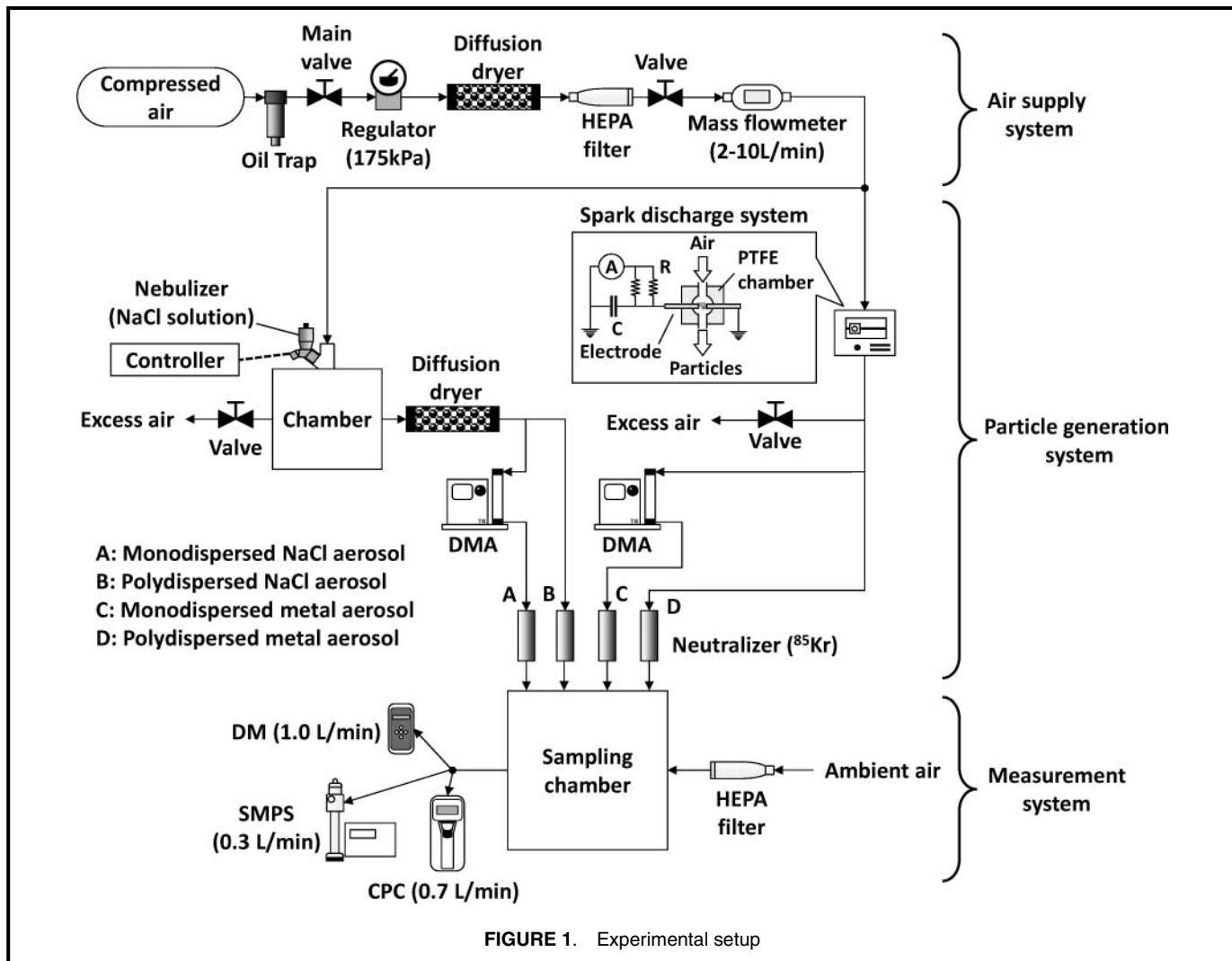
FIGURE 1. Experimental setup
