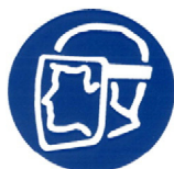
Fig. 2. Example of a precautionary pictogram for individual protection measures. This pictogram represents a face shield (United Nations, 2009a).
