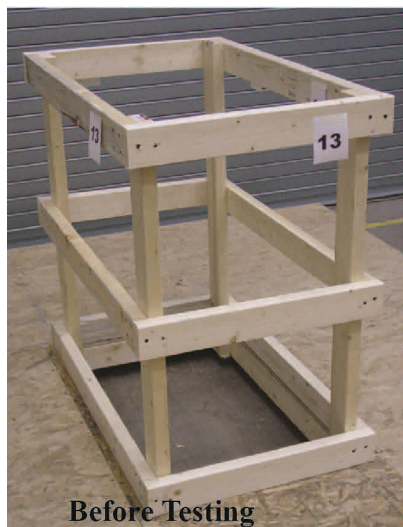
Figure 8. Subject #13 PTF Testing Results Using Screw Fasteners
