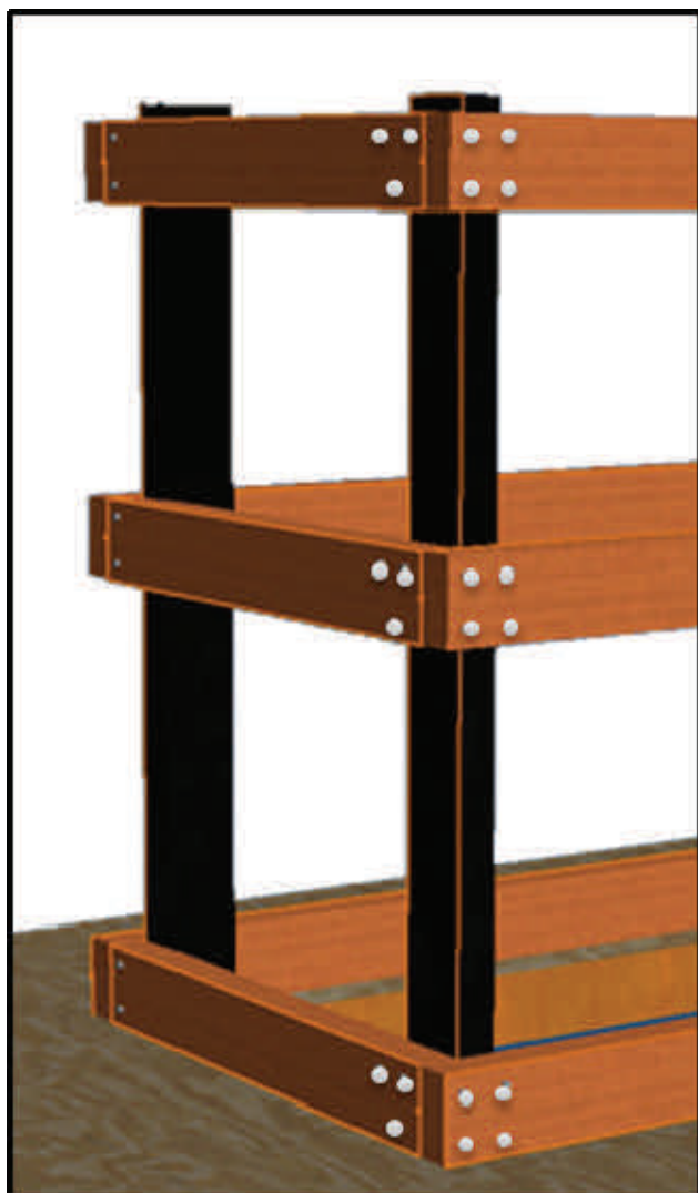
Figure 11. Overlapped Rails and Fastener Placement
