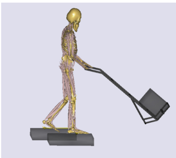
Fig. 2. A cart pushing model developed using AnyBody modeling system.
