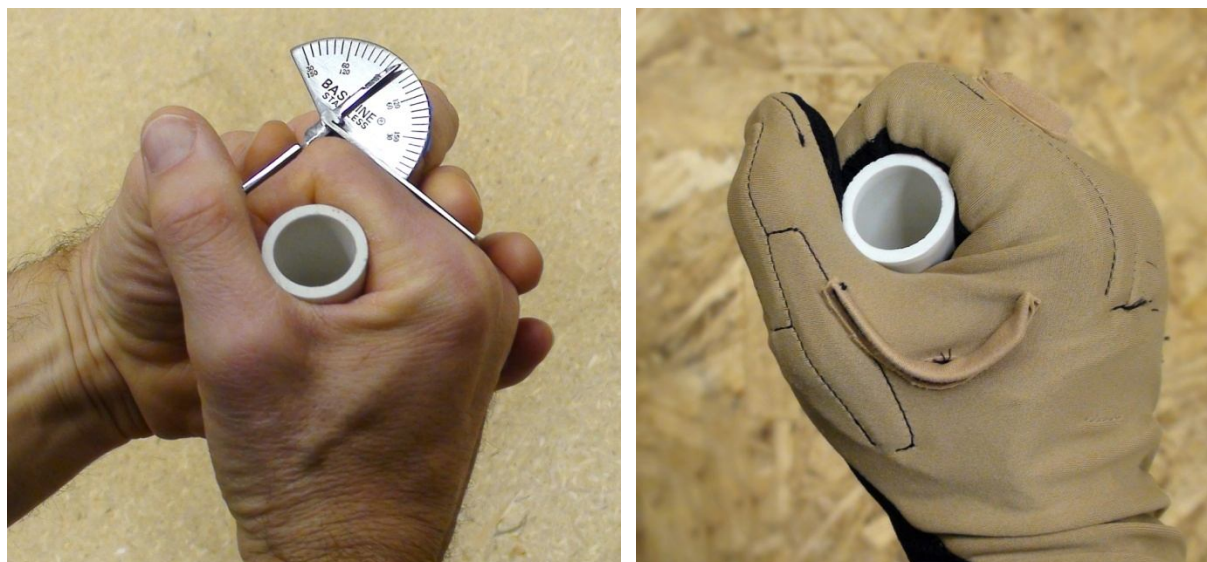
Figure 2. Manual goniometric measurement of the proximal interphalangeal (PIP) joint angle (left), for calibration of the CyberGlove (shown on right).
