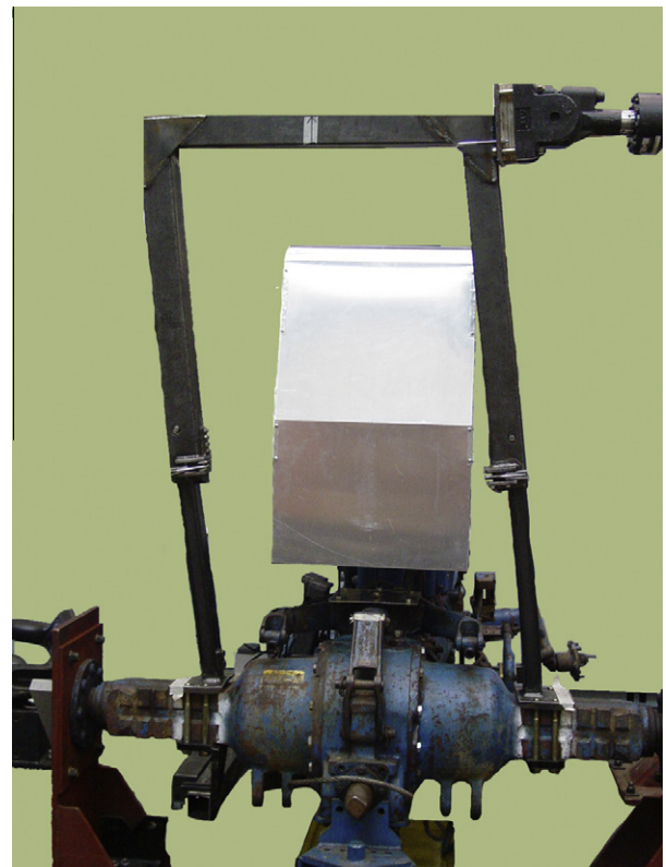
Fig. 5. Typical side load application.
