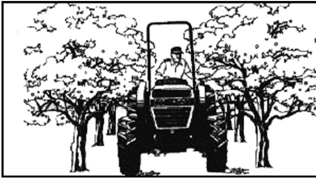
Fig. 1. Factory ROPS mounted on the tractor.
