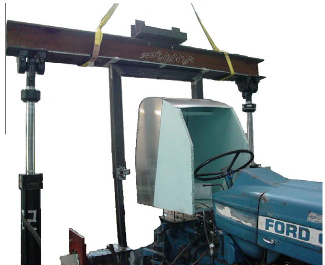
Fig. 4. Vertical crush application.
