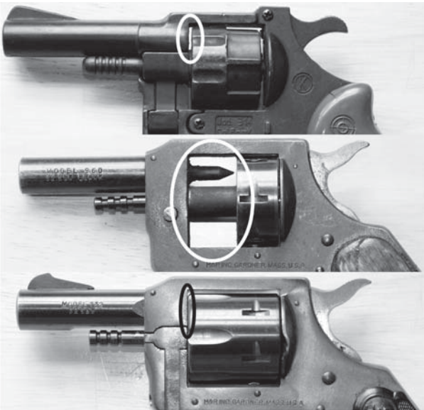
Figure 3. Side view of Kimar .22 starter pistol (top), H&R .32 starter pistol (middle), and H&R .32 revolver (bottom). Circled areas highlight the space between the cylinder and the barrel. In combination with a blocked barrel, the Kimar .22 and H&R .32 starter pistols have a significant gap between the cylinder and barrel, yielding a pathway for gasses to exhaust to the side. The H&R revolver has a very tight fit of the cylinder and the barrel, yielding negligible gap.
