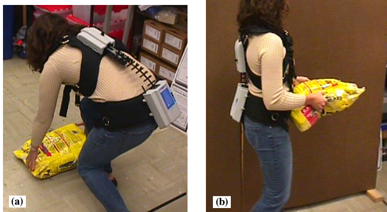
Figure 8. The typical feed handling task, which required subjects to (a) lift each bag and (b) carry it to a designated location.
