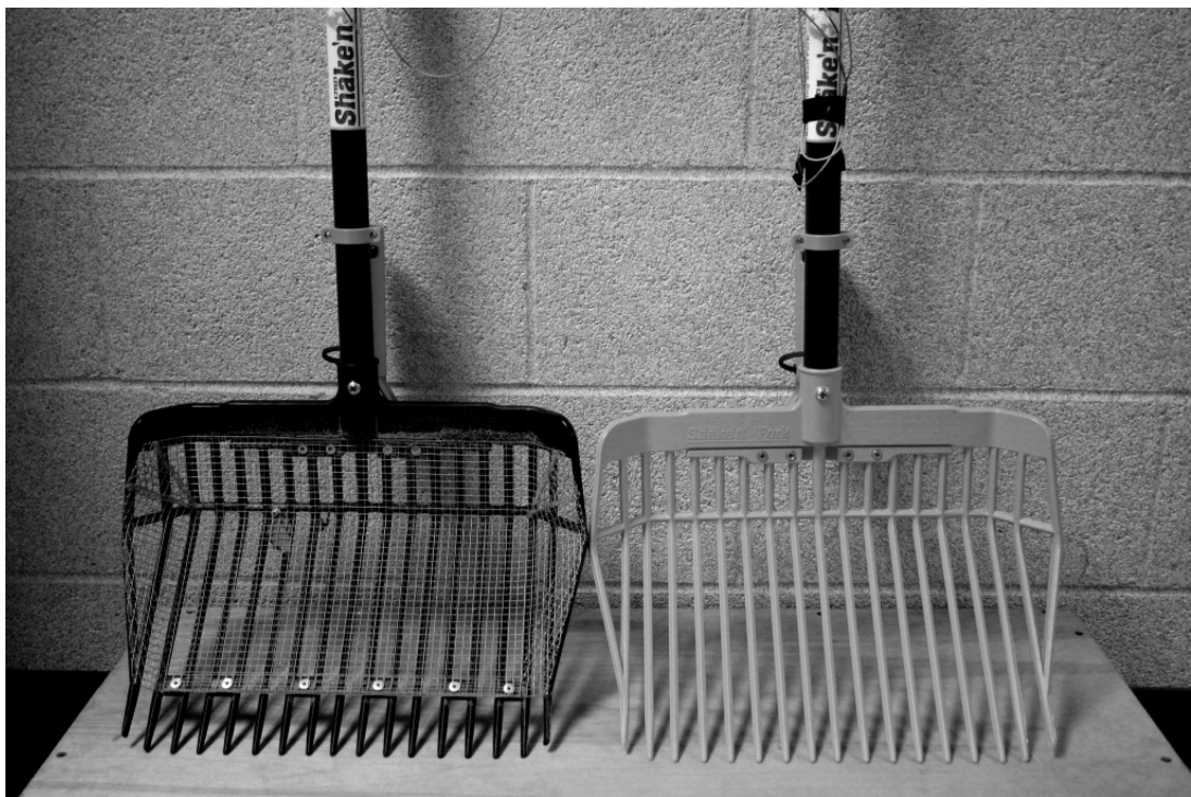
Fig. 2. The two interchangeable baskets evaluated in the study. The black version on the left featured a wire screen (6-mm mesh) for sifting finer material.
