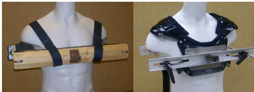
Fig. 1. (Left) Wooden chest harness and (right) plastic chest harness.
