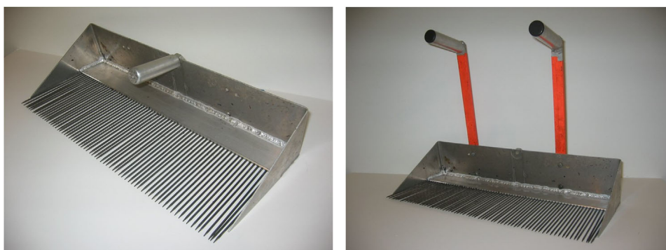
FIGURE 2. Photos of the traditional short-handle blueberry rake (left) and long-handled rake (right). [Color figure can be seen in the online version of this article, available at http://wileyonlinelibrary.com/journal/ajim ]
