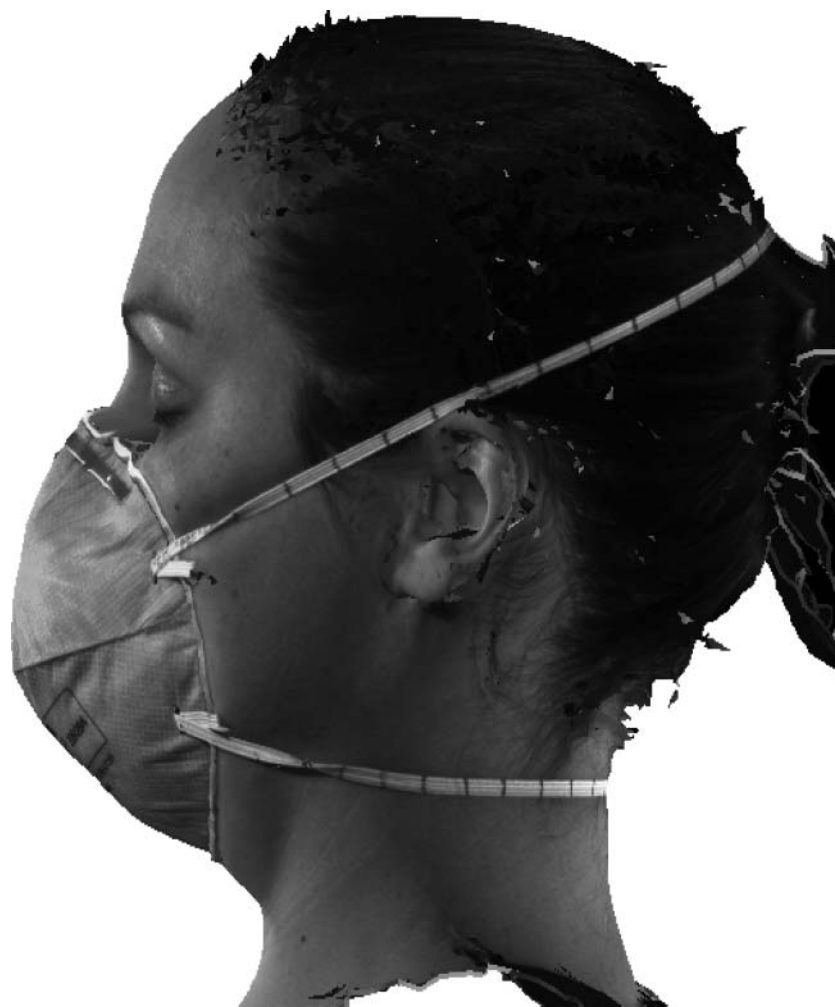
FIGURE 2. Test subject wearing an N95 filtering facepiece respirator with tethering straps marked in one centimeter increments
