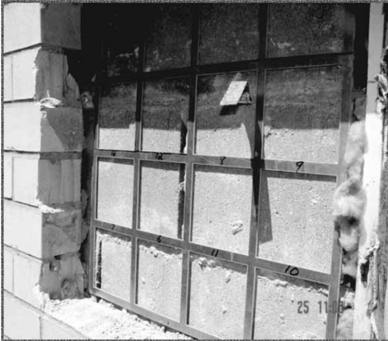
FIG. 3—Sampling template with equal 100-cm 2 sample areas positioned in 18-in. by 18-in. opening in brick veneer.
