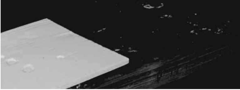
FIG. 1—Original nail-indented surface (dark wood) with its final painted (white) specimen, Number 1, on top.
