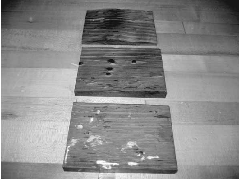
FIG. 3—High-density plastic dies of the three specimens (top to bottom: Spec 2, heavily grooved floor; Spec 1, nail-indented window sill, Spec 3, contoured window sill).
