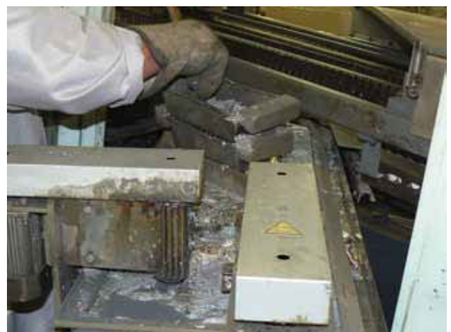
FIGURE 1. Employee cleaning solder dross from a wave solder machine.
