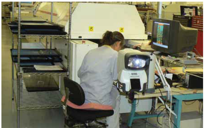
FIGURE 2. Employee inspecting boards near local exhaust of a reflow oven.
