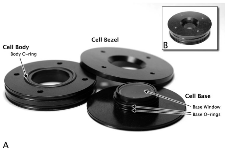
Fig. 1. (A) Permeation cell components. (B) Inset showing assembled permeation cell (without test material or solid media). Prior to assembly, solid medium is placed on top of the base window and test material is held in place between the body and bezel using four screws. The base is then connected to the body/bezel, providing close contact between the solid media and test material and a leak-proof seal. The test material is exposed to clear coat through a 2.54-cm (1 inch) diameter opening in the cell.
