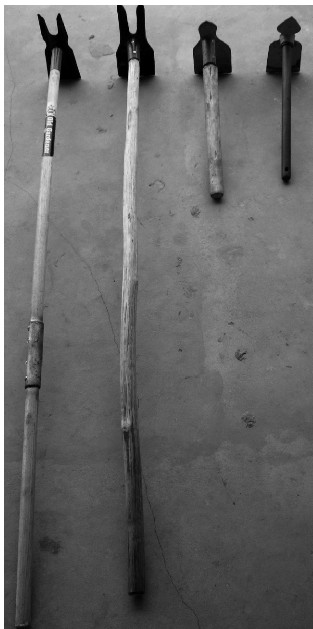
The handle of the model long-handled hoe was cut for shipping to The Gambia and was rejoined with a silver metal tube.
