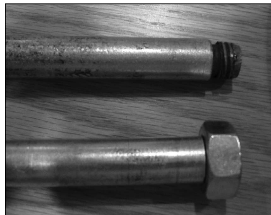
FIGURE 8. Defective ROPS mounting bolts.
