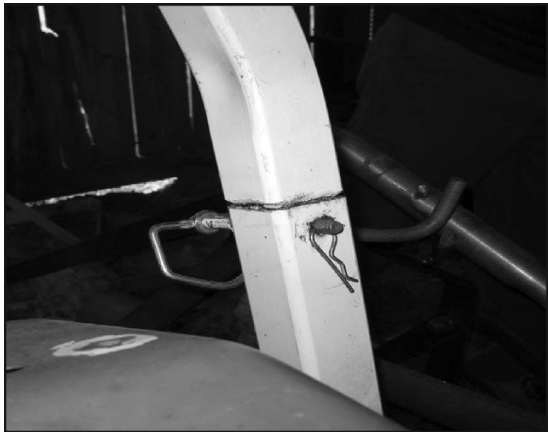
FIGURE 3. ROPS installed on a Satoh 650G that has been cut and pinned together.
