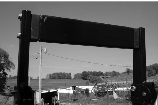
FIGURE 4. Foldable ROPS installed with solid steel extensions (red).
