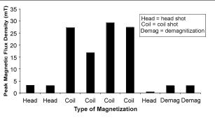
Fig. 2. Successive magnetic field measurements during inspection process of one turbine shaft.
