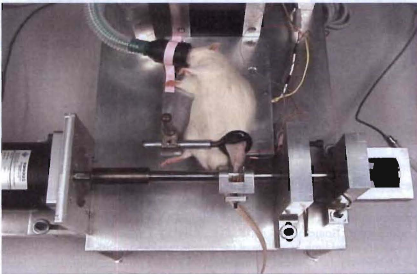
Figure 5. In Vivo dynamometer with an anaesthetized rat on the heated X-Y positioning table. The left foot is secured in the load cell fixture and the knee is secured in 90° flexion.
