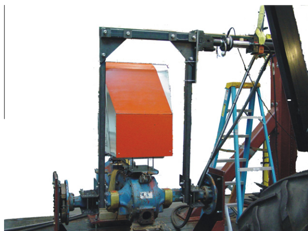
Fig. 5. SAE J2194 transverse loading of Ford-3000 CROPS.
