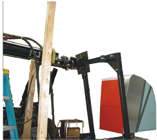
Fig. 3. SAE J2194 longitudinal loading of Ford-3000 CROPS.
