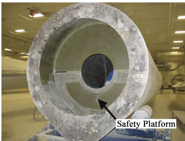
Fig. 4. Safety Platform glassed in as a disk shaped fiberglass part near the root of the wind turbine blade.
